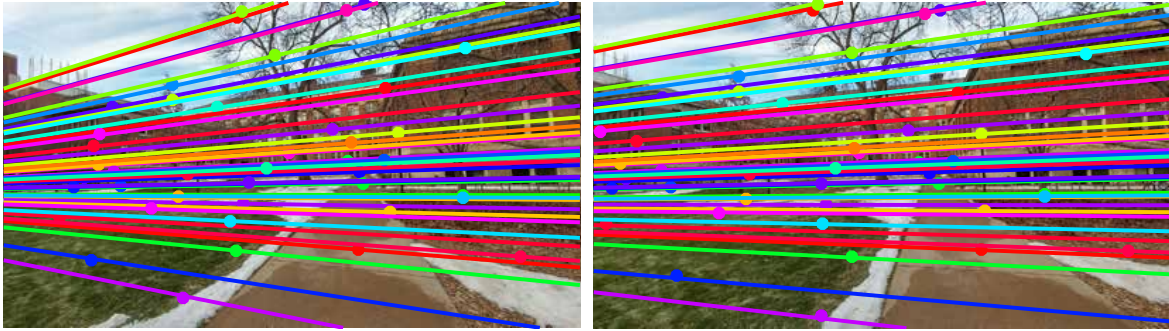
Figure 3: Given matches, you will compute a fundamental matrix to draw epipolar lines.
